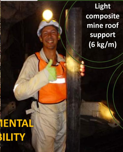
Light composite mine roof support (6 kg/m)
